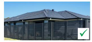
ROOFS – gable or hipped roofs are to be a minimum of 22.5 degrees pitch and skillion roofs a minimum of 10 degrees pitch. Roof materials are to be concrete tiles (flat profile preferred) or metal Colorbond Custom Orb. Roof colour is to be of a natural earth tone with a preference for dark 'grey' tones.
